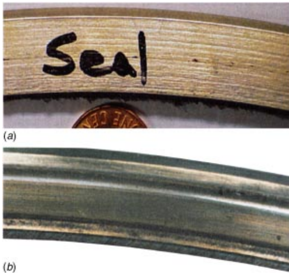
Fig. 12 (a) Previous version of a seal from the engine after about 1000 cycles; (b) new and improved version of the seal after 2000 cycles at the same location on the similar engine
